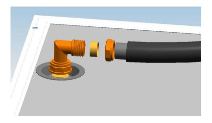
3. Assemble 3/4" moufa to the outside thread connector which is on the other side of collector. Then assemble the short PEX Black Pipe and Thermal Insulation Pipe.
